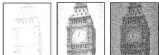
Fig. 4. Visual images of Big Ben on a 256 gray scale with spatial resolution of 256 by 256 pixels. The original photograph is suppressed beneath a threshold of \Delta_0 = 30 . Noise from Gaussian distributions is added to the gray scale values in each pixel. Left-to-right the standard deviations of the noise are \sigma = 10, 90 and 300 , respectively. The information content in each pixel is 1 bit: if the gray scale value in that pixel is greater than threshold (30) the pixel is painted black. Otherwise it remains white. Reproduced from Simonotto et al. (1997), with permission.
